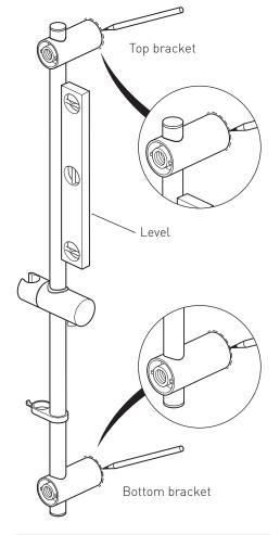
Find the centre of the marked position. Suitably fix the wall bracket to the wall using appropriate fixings.
