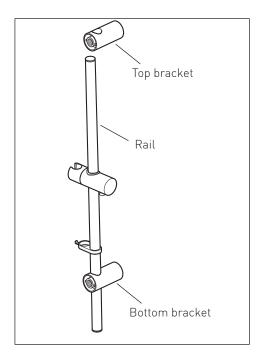
Push a rubber insert into the hole of the bracket, screw in the grub screw and tighten.
