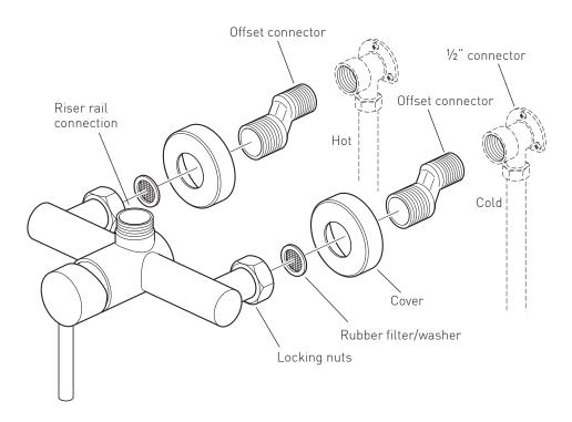
Before installing your new mixer, flush through the pipe work to ensure removal of debris, turn off the water supply.
