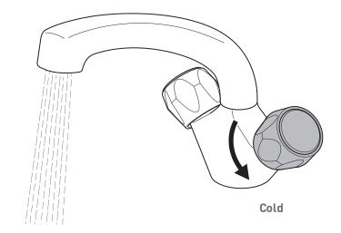
Turning the handle anti-clockwise will decrease the water temperature.
