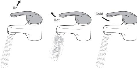
Moving the mixer lever upwards will increase the flow of water.
