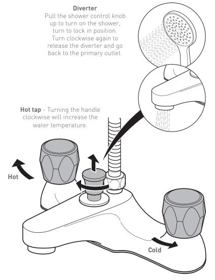
**Cold tap** - Turning the handle anti-clockwise will decrease the water temperature.
