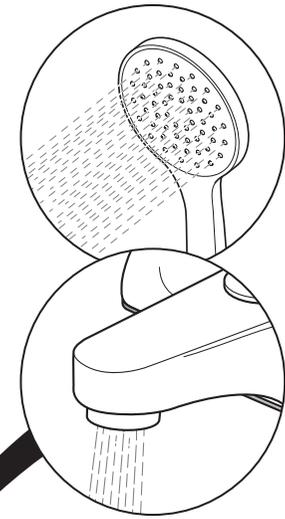
**Hot tap** - Turning the handle clockwise will increase the water temperature.
