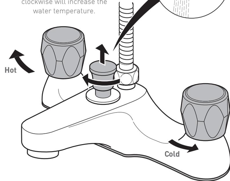
**Cold tap** - Turning the handle anti-clockwise will decrease the water temperature.
