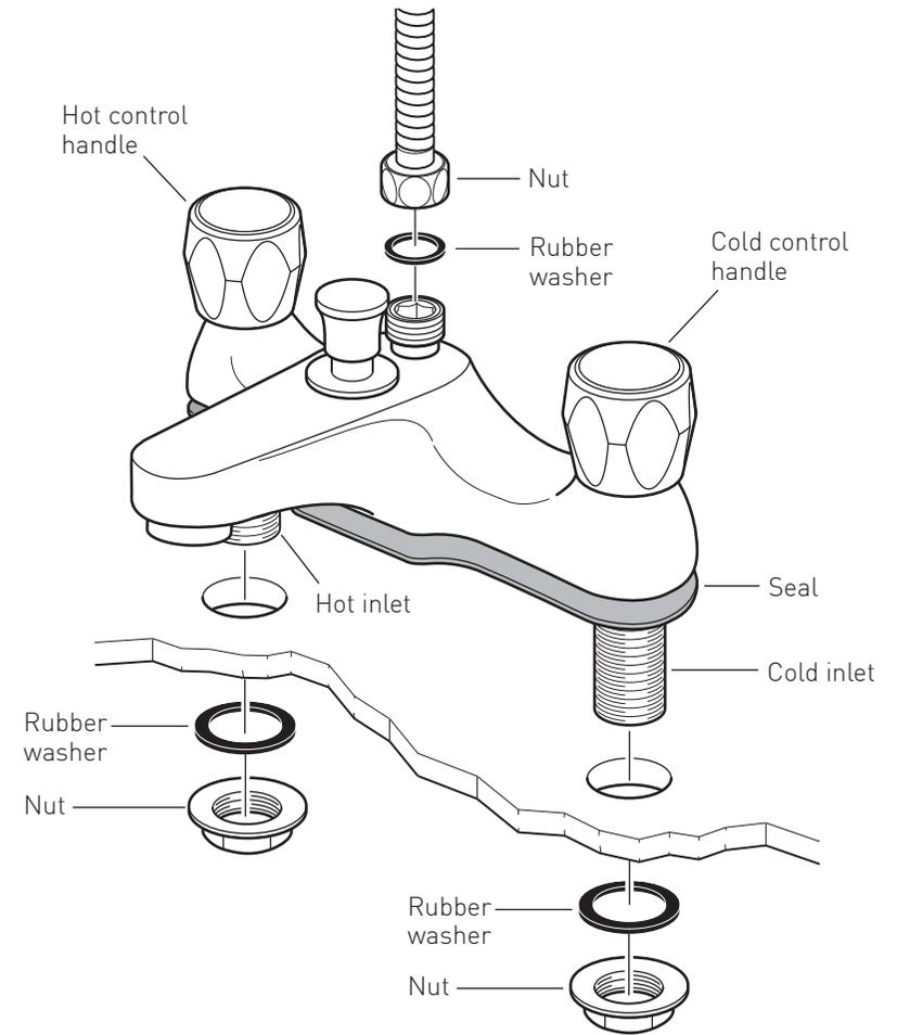
Before installing your new mixer, flush through the pipework to ensure removal of debris, turn off the water supply.
