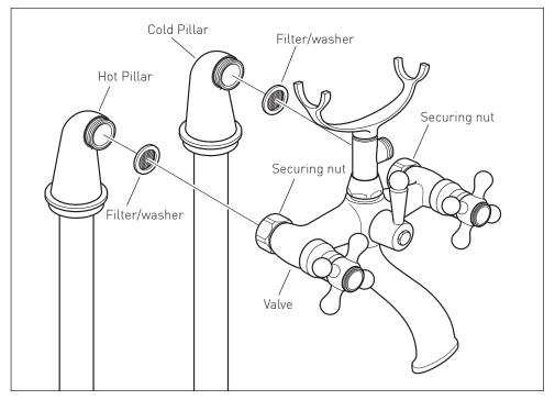
Push a filter/washer into both securing nuts on the mixer.
