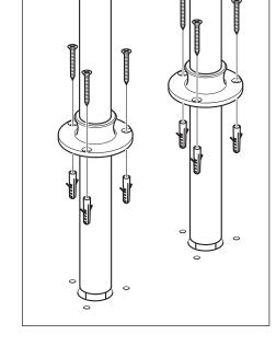
Tighten all 3 grub screws on each foot plate to lock the support tubes in position use the supplied hex key.
