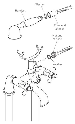
Place one of the rubber washers into the cone end of the hose and screw to the handset.
