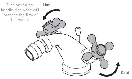
Turning the cold handle anti-clockwise will increase the flow of cold water.
