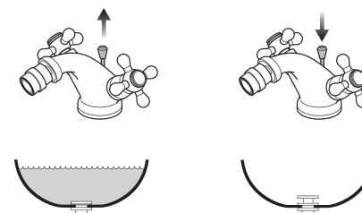
Pull the waste control rod up to close the plug and fill the basin.
