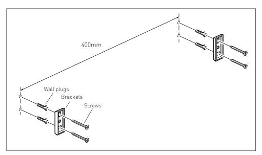
Remove the two brackets from the back of the shelf by releasing the two grub screws. The brackets should be set apart by **400mm** (see above). Position the brackets, mark the four fixing points making sure the brackets are level. Drill the holes using a suitable 6mm masonry drill bit to a suitable depth for the wall plugs and secure with supplied screws, making sure brackets are level.
