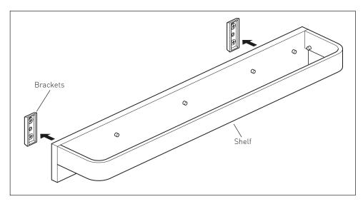
Offer the shelf to the brackets, making sure that the grub screws on the underside line up with the brackets.
