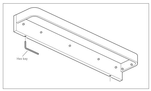
With the shelf against the wall tighten both grub screws on the underside using the supplied hex key.
