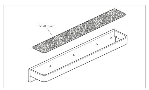
Finally place the shelf insert into the body to rest on the internal pins.
