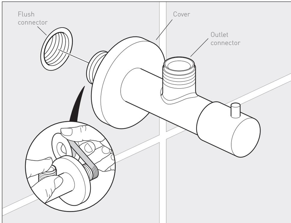
Using PTFE tape on the thread screw the valve into the connector. Make sure that the outlet is pointing upwards.
