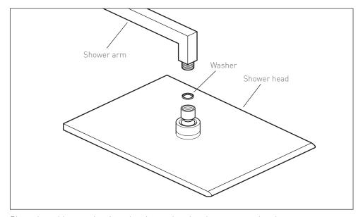
Place the rubber washer into the shower head and screw onto the shower arm. The shower head can be tilted to the required position.
