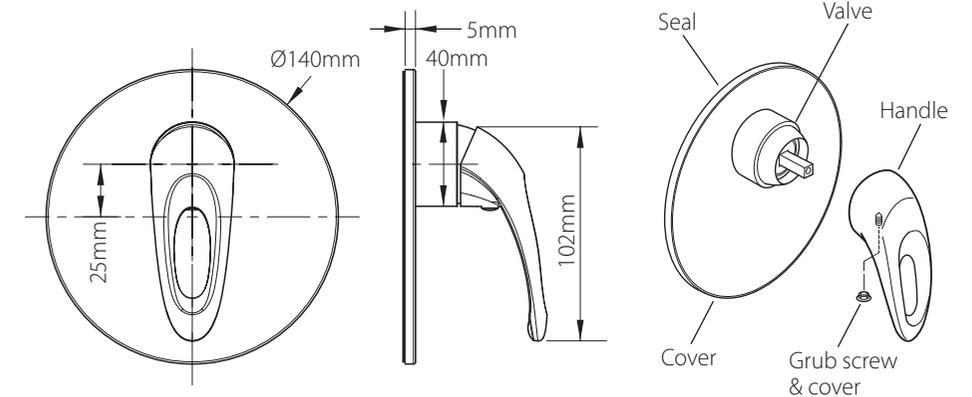
Remove the backing paper from the seal on the back of the cover. Slide the cover over the valve, push onto the wall until it makes contact.
