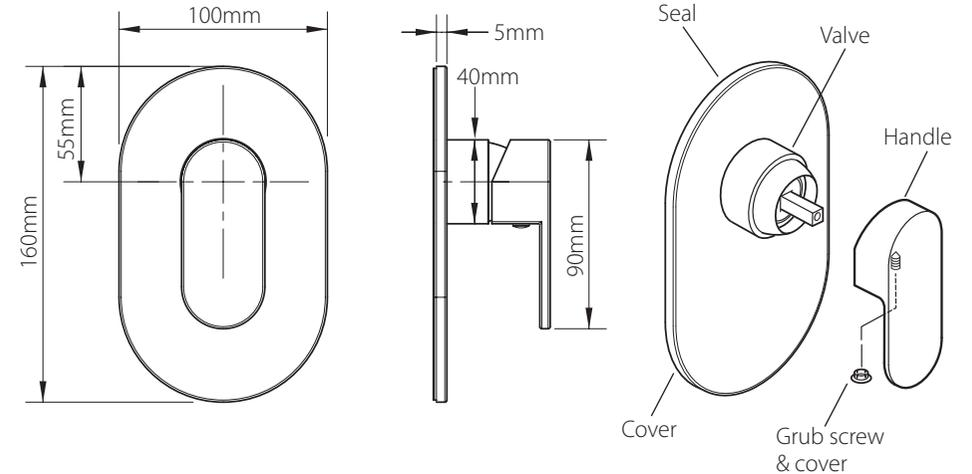
Remove the backing paper from the seal on the back of the cover. Slide the cover over the valve, push onto the wall until it makes contact.
