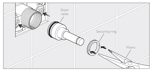
Close both non return valves. Remove the speedfit connector. Using a pair of long-nosed pliers unscrew the securing ring and remove.
