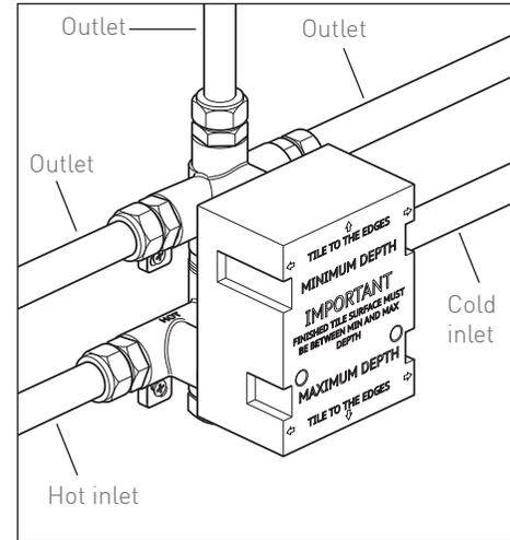
Use the supplied adaptors if required. Connect hot supply to the lower left inlet of the valve and cold supply to the lower right inlet. Connect the top and bottom outlets to the desired channels.
