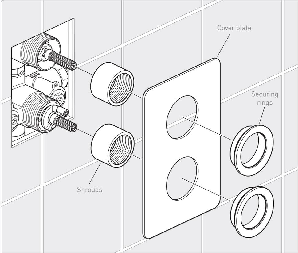
Screw shrouds on ensuring they sit proud of the finished wall. The shrouds can be turned/adjusted to achieve this.
