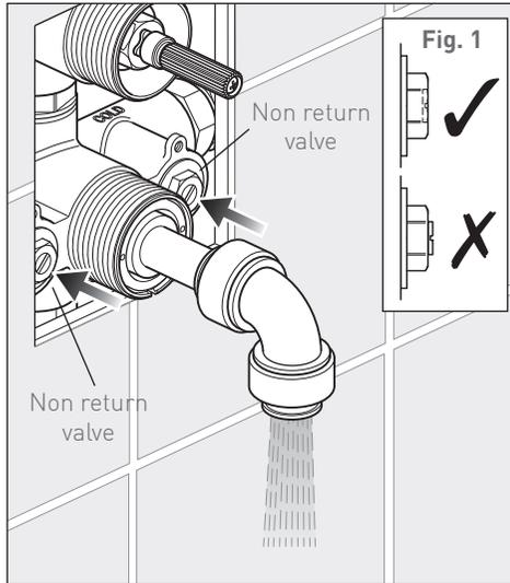
Turn on at the mains, open both non return valves and allow the debris and water to drain. When loosening the non return valve do not unscrew further than the face of the nut (**see Fig. 1**). After approximately two minutes of flushing the pipe work and product close both non return valves. Do not overtighten.
