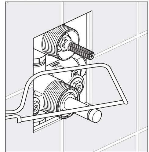
**Important:** ensure the hot and cold water supplies have been isolated. Using a suitable tool, cut the end off the drain through the easy cut section.
