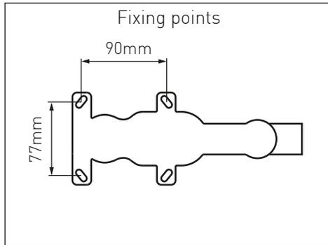
Select the position for the shower valve and offer the shower valve to the wall, make sure the valve is vertical with a level and mark the 4 fixing points with a suitable pencil, see above left for dimensions. Remove the shower valve from the wall, drill the holes to a suitable depth for the wall plugs and secure with suitable screws.
