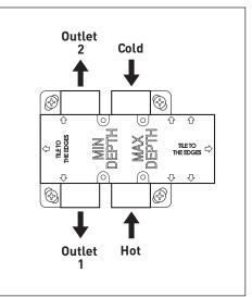
Finish the wall by tiling up to the mortar guard, keep the final finished wall surface between the min and max marks.
