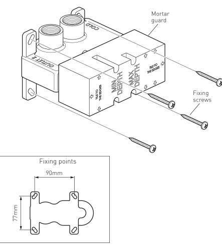
Select the position for the shower valve and offer the shower valve to the wall, make sure the valve is horizontal with a level and mark the 4 fixing points with a suitable pencil, see above left for dimensions. Remove the shower valve from the wall, drill the holes to a suitable depth for the wall plugs and secure with suitable screws. Installation - Quick guide
