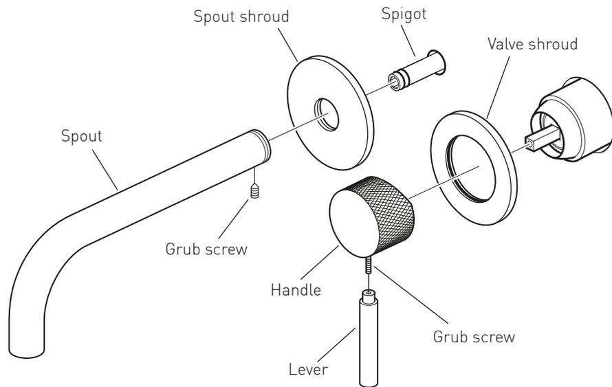
Slide the shroud over the valve, push onto the wall until it makes contact.
