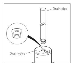
Turn on at the mains, and allow the debris and water to drain.
