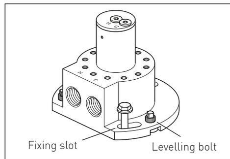
Connect the hot and cold supplies to the base. The hot should be fixed to the outlet marked **H** and the cold fixed to **C**.
