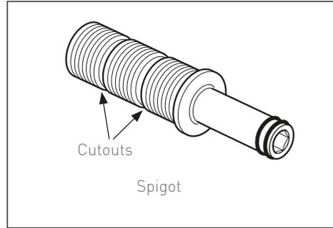
Screw the spigot into a 1/2" female elbow (not supplied) or other suitable connection. Connect the water supply from the valve.
