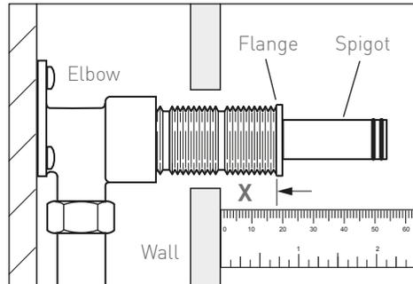
Remove the spigot from the elbow. If necessary carefully cut the bottom of the spigot by this measurement. Remove any burrs.
