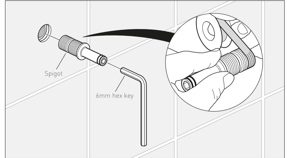
Using PTFE tape on the thread, screw the spigot into the wall and tighten using a 6mm hex key (not supplied).
