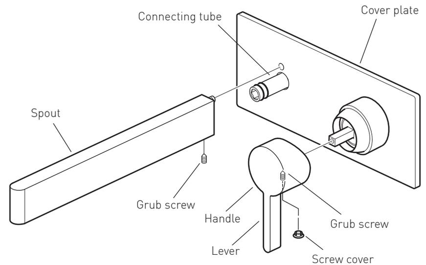
Slide the cover plate over the valve, push onto the wall until it makes contact.
