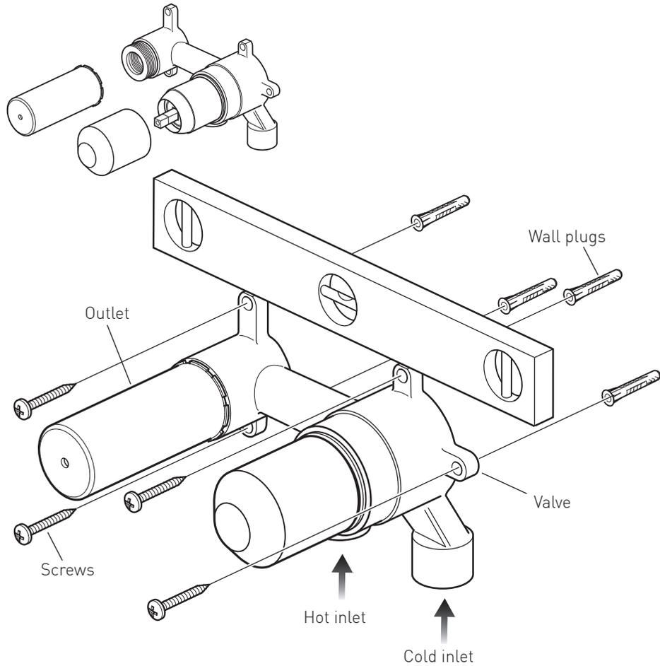
**⚠ Warning!** Please check for any hidden cables and pipes before drilling holes in the wall. Before installing your new mixer, flush through pipework to ensure removal of debris, turn off the water supply.
