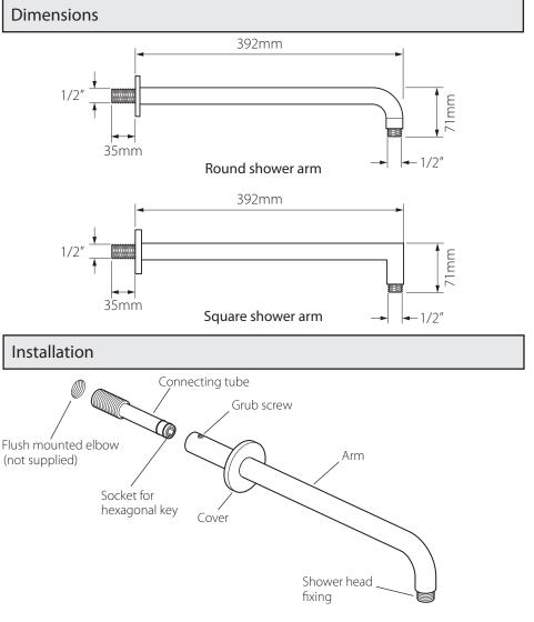
Prepare the end of the pipe work with an  $\frac{1}{2}$ " fixed elbow (not supplied). Fix in the correct position, and flush with the final surface of the wall.
