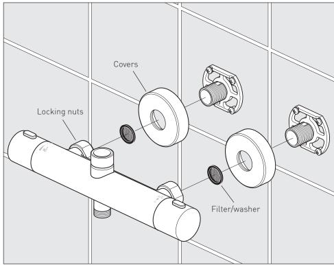
Screw the covers on each offset connector. Place a rubber filter/washer in each of the locking nuts on the valve and screw onto the connectors.
