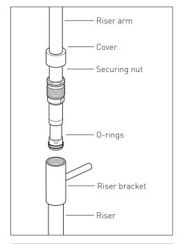
Remove the nut and seal from the top of the valve and slide onto the riser rail. Push the riser onto the connection on the top of the valve, slide down the seal and tighten the nut.
