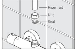
Slide the wall bracket onto the riser bracket.
