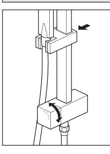
Place the cone part of the hose into the handset holder, the holder can be repositioned by pressing the button at the back and sliding up and down.
