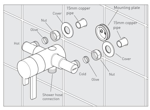
During and after installation protect the outer parts of the valve to avoid damage to plated surfaces.
