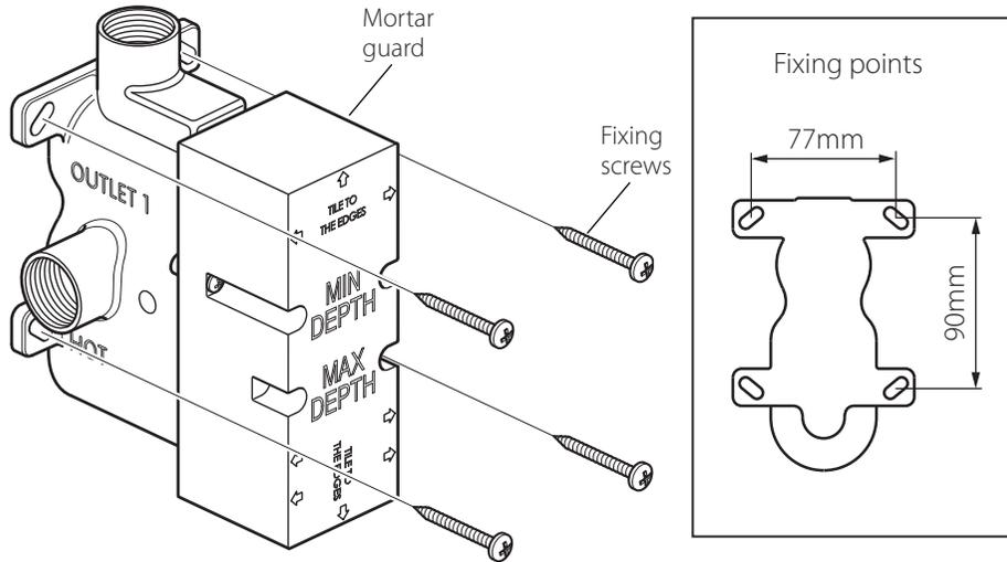
Select the position for the shower valve and offer the shower valve to the wall, make sure the valve is vertical with a level and mark the 4 fixing points with a suitable pencil, see above right for dimensions. Remove the shower valve from the wall, drill the holes to a suitable depth for the wall plugs and secure with suitable screws.
