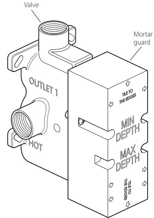
Rinse pipe work thoroughly before fitting the valve: do not allow dirt, metal particles or shavings to block the filters fitted on inlets.
