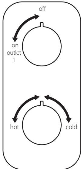
Turning the bottom handle anti-clockwise will increase the water temperature.
