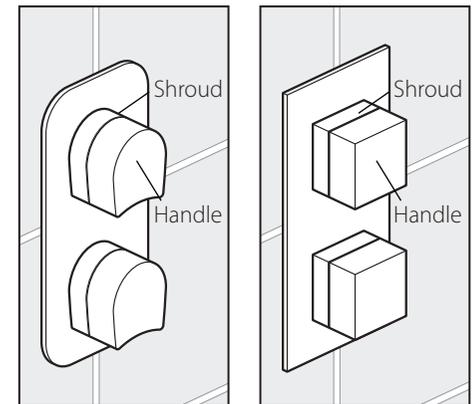
**Please note:** if the handle/shroud assemblies do not align, remove the offset spline and replace the other way up.
