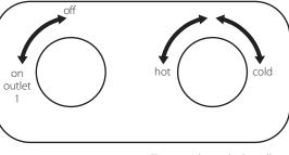
Turning the right handle anti-clockwise will increase the water temperature.
