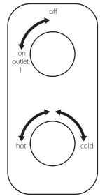
Turning the left handle controls the flow of water to the outlet.
