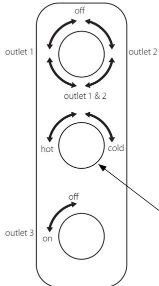
Turning the left handle controls the flow of water to the outlets.
