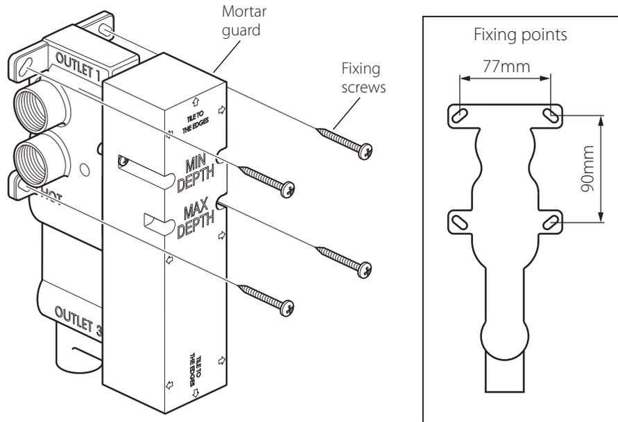
Select the position for the shower valve and offer the shower valve to the wall, make sure the valve is vertical with a level and mark the 4 fixing points with a suitable pencil, see above right for dimensions. Remove the shower valve from the wall, drill the holes to a suitable depth for the wall plugs and secure with suitable screws.
