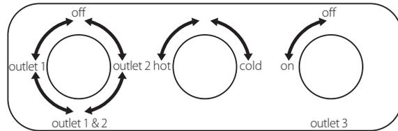
Turning the right handle controls the flow of water to the outlet.
