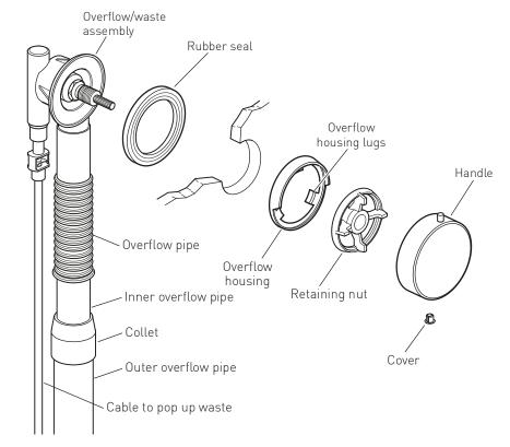
The length of the overflow pipe can be adjusted by pulling apart or pushing together the inner and outer overflow pipes.
