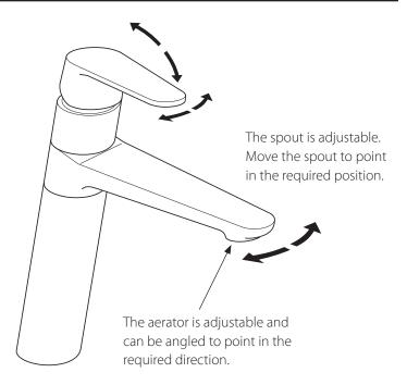
Moving the mixer lever upwards/downwards will increase/decrease the flow of water. Moving the mixer lever from right to left will increase the water temperature.
