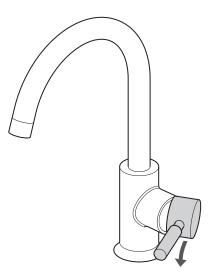
Moving the mixer lever forwards will increase the water temperature.
