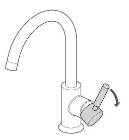
Moving the mixer lever to the right will increase the flow of water.
