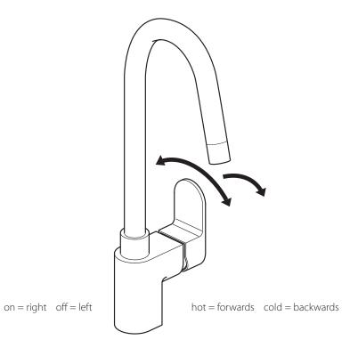
Moving the mixer lever to the right will increase the flow of water.
