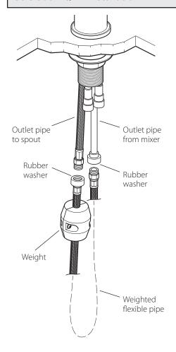
Connect the flexible pipe with the weight at the end to the flexible pipe coming from the mixer. Make sure that the rubber washer is in place within the nut.
