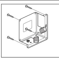
Make sure that the rubber washers are in place in the flexible pipes. Connect the flexible pipe from the tap to the bottom outlet marked 'Outlet'. Connect the other flexible pipe to the side connection marked 'Inlet'.
