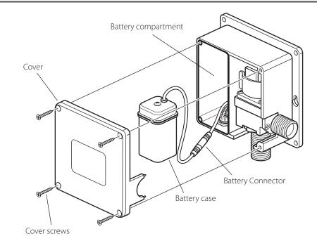
The unit is supplied with a battery backup. Should the mains supply fail and the tap still will not function then the batteries may need replacing. Before installing the control box on the wall fit the supplied batteries as follows.
