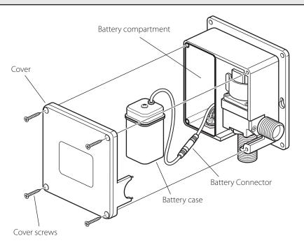
The unit is supplied with a battery backup. Should the mains supply fail and the tap still will not function then the batteries may need replacing. Before installing the control box on the wall fit the supplied batteries as follows.
