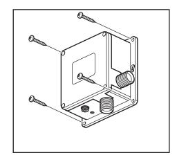
Make sure that the rubber washers are in place in the flexible pipes.
