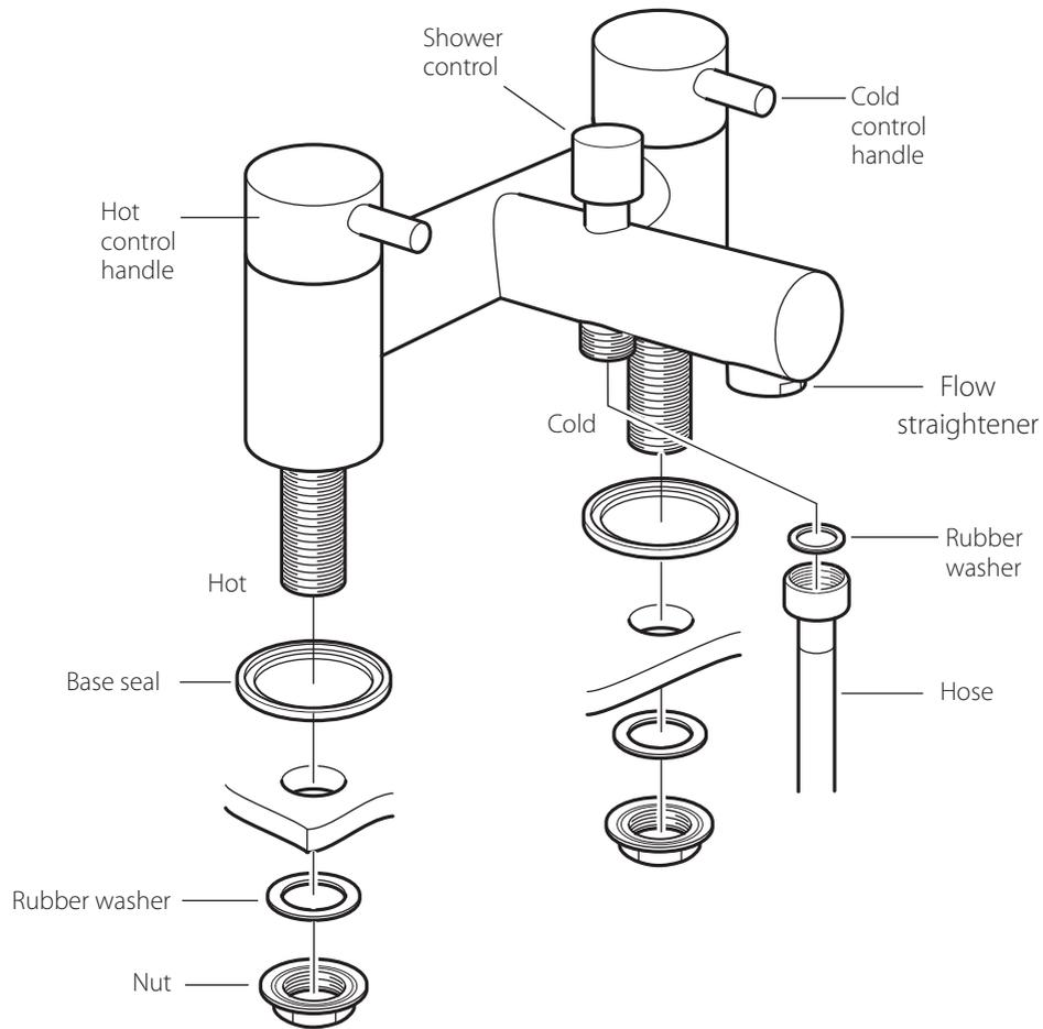
Before installing your new mixer, flush through the pipework to ensure removal of debris, turn off the water supply.
