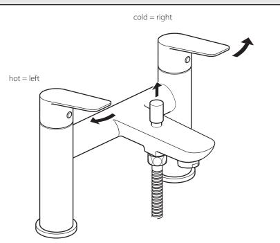
Moving the levers in the direction of the arrows will increase the flow of water. Pull the diverter knob up to turn on the shower.
