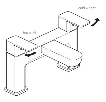
Moving the levers in the direction of the arrows will increase the flow of water.
