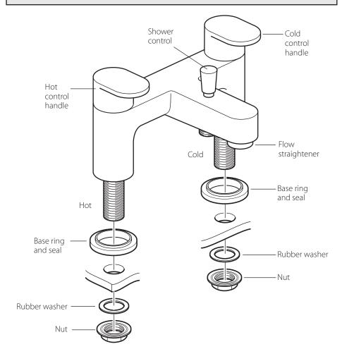
Before installing your new mixer, flush through the pipework to ensure removal of debris, turn off the water supply.
