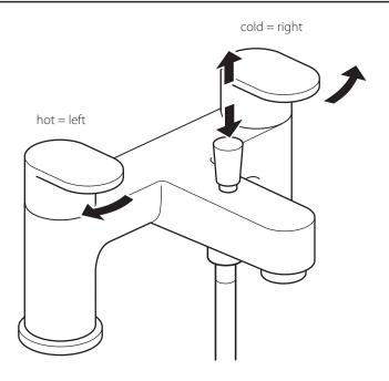
Moving the levers in the direction of the arrows will increase the flow of water. Pull the shower control knob up to turn on the shower, push down to close.
