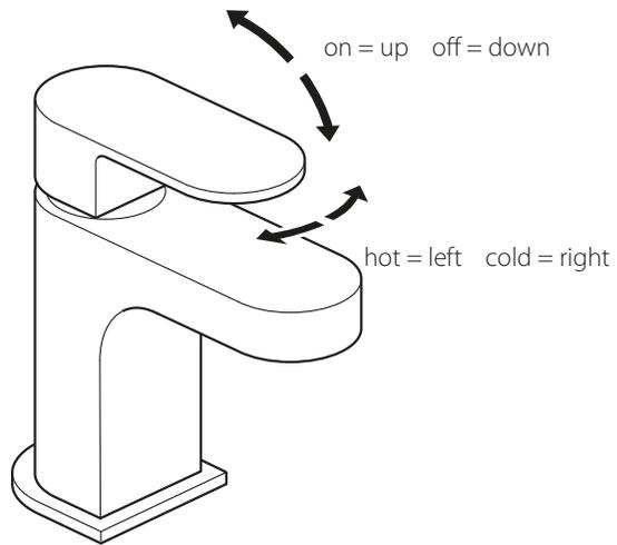
Moving the mixer lever upwards/downwards will increase/decrease the flow of water.
