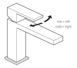
Moving the mixer lever from right to left will increase the water temperature.
