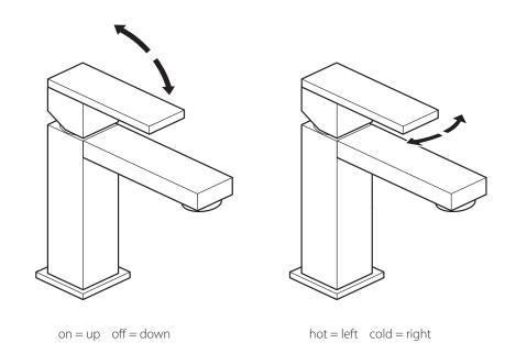
Moving the mixer lever upwards/downwards will increase/decrease the flow of water. Moving the mixer lever from right to left will increase the water temperature.
