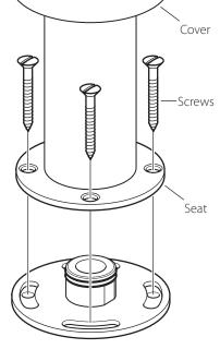
Position the seat/body on the floor in the correct orientation for the spout, mark the 4 fixing holes and the centre hole. Remove the seat/body.
