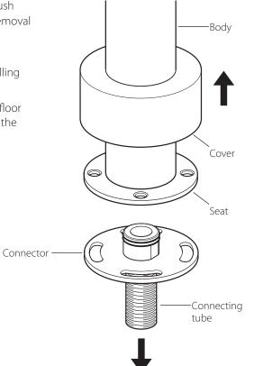
Connect to the water supply using PTFE tape on the thread, screw the connector
