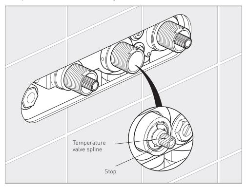
Turn the spline of the thermostatic valve clockwise to decrease the temperature and anti-clockwise to increase the temperature until 38°C is achieved at outlet.
