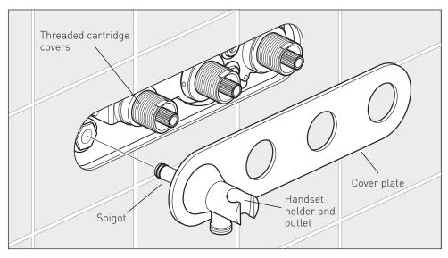
Guide the handset holder with spigot attached partially onto the valve and then slide the cover plate over the threaded cartridge covers. Push on the cover plate and handset holder. Apply a thin bead of silicone around the outside to seal against the tiled surface.
