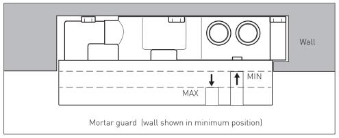
Select the position for the shower valve and offer the shower valve to the wall, make sure the valve is level and mark the 6 fixing points with a suitable pencil, see above for dimensions. Remove the shower valve from the wall, drill the holes to a suitable depth for the wall plugs and secure with suitable screws.
