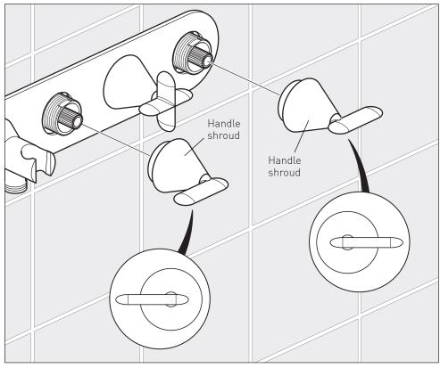
Carefully slide on both control handles onto spline of the valve. While holding the handle in the horizontal position screw the shroud until touches the cover plate.
