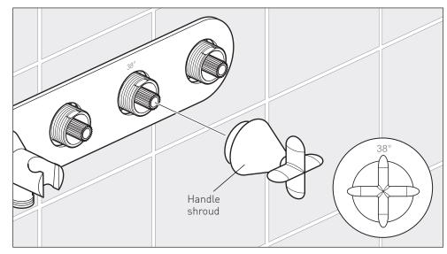
Carefully slide the temperature handle onto the centre spline of the valve. While holding the handle in the vertical/horizontal position screw the shroud until touches the cover plate. The handle is etched to show alignment to the 38°c position on the plate.
