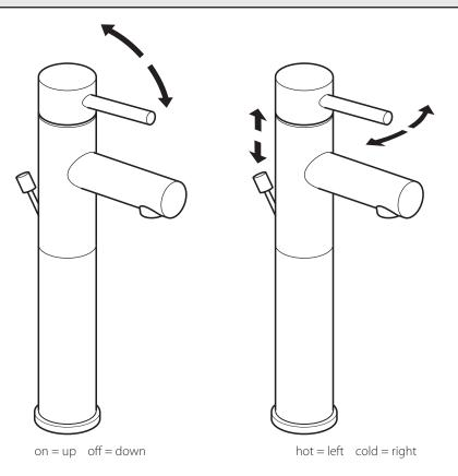
Moving the mixer lever upwards/downwards will increase/decrease the flow of water. Moving the mixer lever from right to left will increase the water temperature. Pull the vertical control rod up to close the waste outlet and push down to open.
