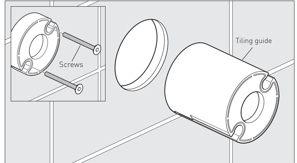
Remove the 2 screws using the suitable hex key provided with the ZON-128 and pullout the tiling guide.
