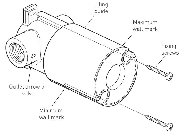
Select the position for the shower valve and offer the shower valve to the wall, make sure the valve is level and mark the 2 fixing points with a suitable pencil. Remove the shower valve from the wall, drill the holes to a suitable depth for the wall plugs and secure with suitable screws.
