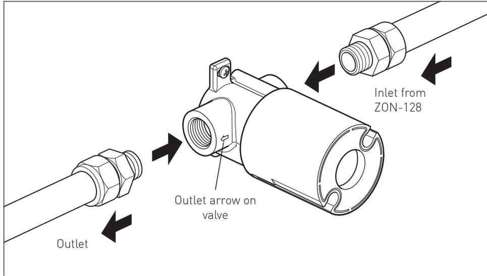
After removing the blanking plug and adding the outlet adaptor to the ZON-128 connect the water supply to the right inlet of the valve. Connect the outlet (arrow on valve) to the desired channel e.g. shower head and handset.
