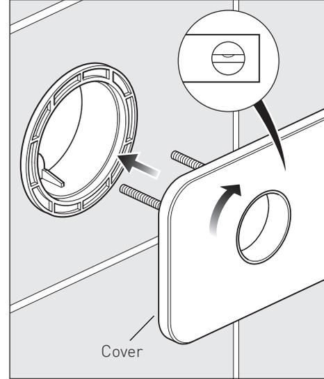
With the correct cover orientation, use the screws to locate the holes in the valve body.
