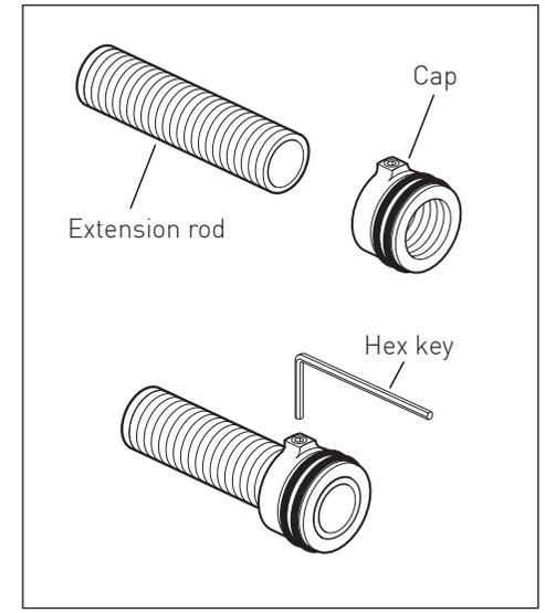
Screw the cap onto the rod until it's flush and tighten the grub screw on the cap using the smaller hex key provided with the ZON-128.
