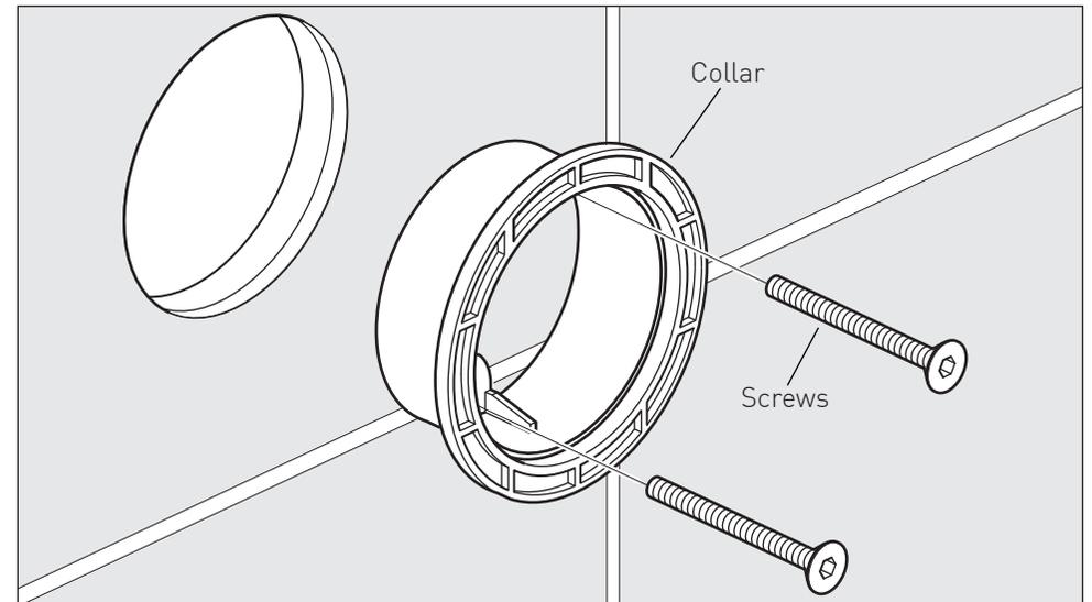
Slide the collar into the hole. Line up the holes and secure in position using the screws from the previous step.
