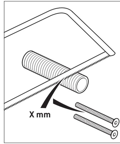
Cut away the measured distance (**X mm**) from the end of the rod as well as the 2 screws provided with the ZON-143 trim.
