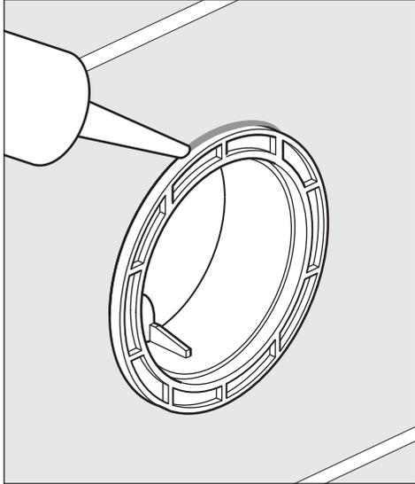
Apply a thin bead of silicone between the collar and the tiles.
