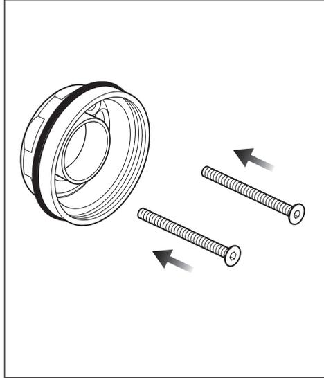
Place the screws inside the fixing nut on opposite sides
