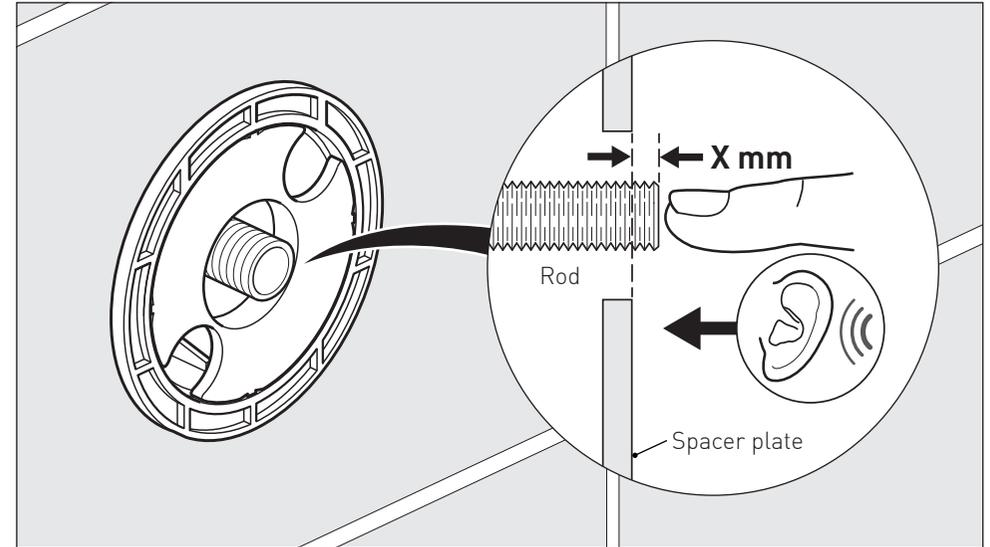
Measure the distance (**X mm**) the rod protrudes from the level of the spacer plate and then unscrew the rod and remove the spacer plate. **Note:** Ensure the cartridge is pushed in (the off position).
