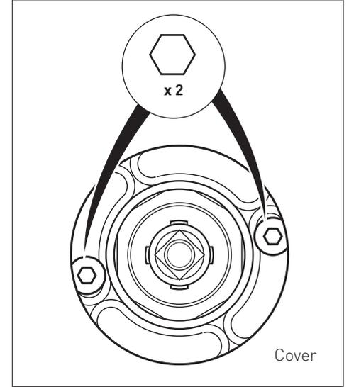
Make sure the cover is level and tighten the screws using the suitable hex key provided with the ZON-128 to secure the cover.
