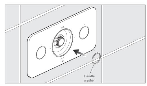
The handle washer is then placed over spline adapter.
