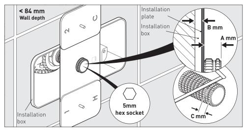
Measure the distance between the installation plate and the end of the spline adapter **(A mm)**. Measure how far the installation box protrudes from the wall **(B mm)** and plus that to  $\mathbf{A} = \mathbf{C}$ . Remove the installation plate. Remove the spline by using a 5mm hex key in the centre of the spline adaptor. Cut down the spline adapter to the required measurement **(C mm)** using a hacksaw, remove any burrs. Screw the spline back in.
