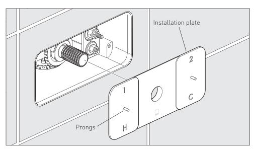
Remove the installation plate using the prongs.
