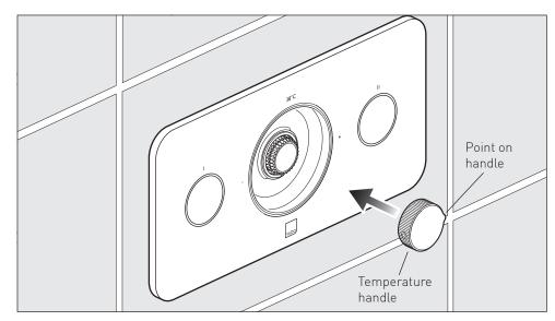
Use the handle to fully rotate the spline clockwise. Lift off the handle, and locate it onto the spline adapter so the point is facing the +.
