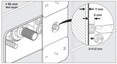
Ensure the extenders are pushed inwards so that the cartridge is in the off position. Measure to the end of the button extender (X mm). Measure how far the installation box protrudes from the wall (Y mm) and plus that to (X mm) = Z mm.
