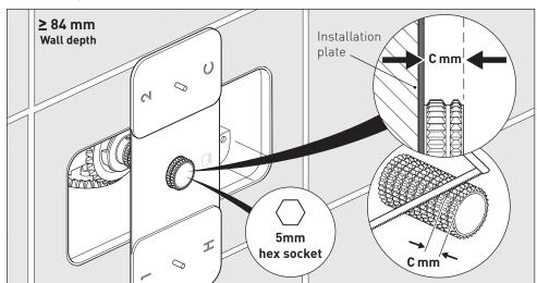
Measure the distance between the installation plate and the end of the spline adapter **(C mm)**. Remove the installation plate. Remove the spline by using a 5mm hex key in the centre of the spline adaptor. Cut down the spline adapter to the required measurement **(C mm)** using a hacksaw, remove any burrs. Screw the spline back in.
