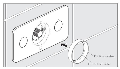
The friction washer is then placed into the central hole of the plate, make sure that the lip is on the inside.
