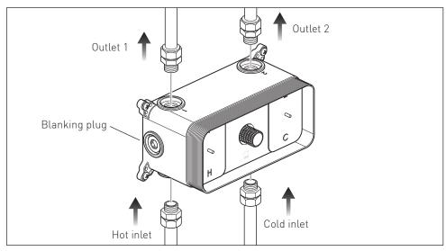
Connect hot supply to the lower left inlet of the valve and cold supply to the lower right inlet. Connect the outlets to the desired channels e.g. shower head and handset. If using an additional module, remove a blanking plug on the desired side using a 12mm allen key.
