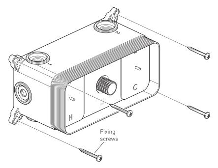
Select the position for the shower valve and offer the shower valve to the wall, make sure the valve is level and mark the 4 fixing points with a suitable pencil. Remove the shower valve from the wall, drill the holes to a suitable depth for the wall plugs and secure with suitable screws.
