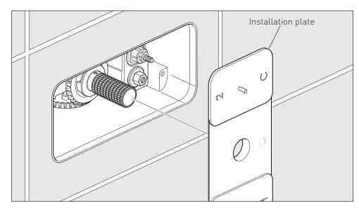
Rotate the installation plate 90° and slide over the spline adapter until it makes contact with the wall.
