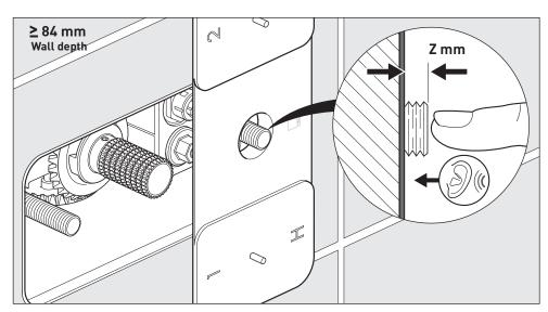
Ensure the extenders are pushed inwards so that the cartridge is in the off position. Measure to the end of the button extender.
