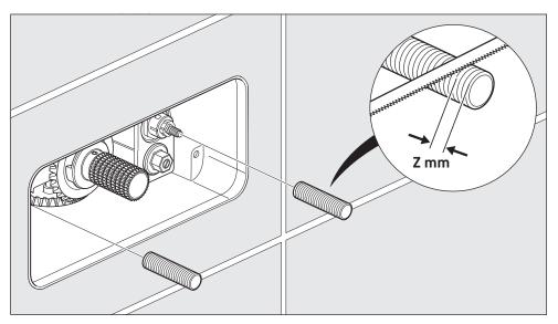
Remove the extenders. Trim the extenders as per the measured distance (Z mm).
