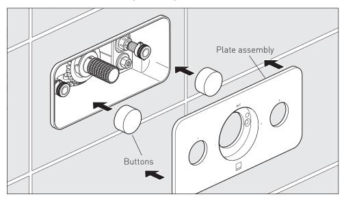
Place the buttons onto the caps and offer the plate up to the wall. Without fixing the plate, check if when both buttons are installed whether they sit flush with the plate. If not, adjust screw cap or trim more of the extender.
