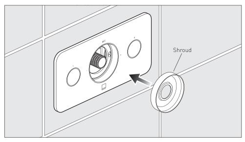
The shroud is then placed into the friction washer.
