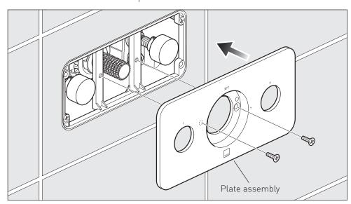
The plate assembly is then located over the middle spline and using the two small screws it is secured to the trim plate.
