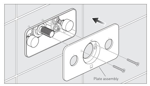
Use the two longer screws to secure the plate assembly to the valve using the two top holes on the plate.
