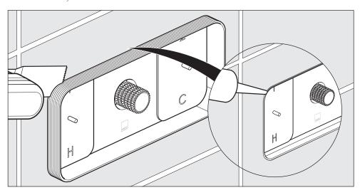
Using the box of the valve as a guide, tile around the box as tight as possible. Carefully cut around the box of the valve using an appropriate tool, ensuring you leave a smooth, even edge, flush with the wall. For installation < 84 mm the installation box may protude up to 4mm from the wall. Do not cut beyond the ribbed section.
