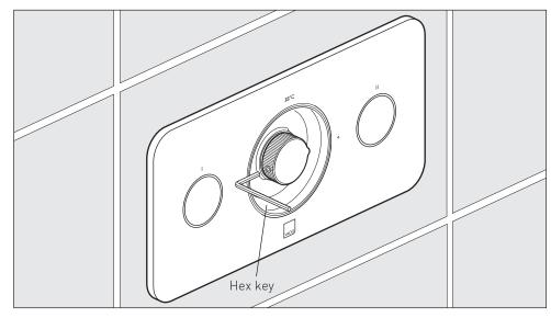
Using the supplied hex key, tighten the grub screw on the side of the handle.
