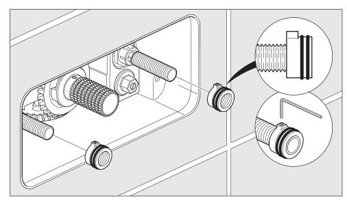
Replace extenders. Add the screw caps from the button connection kit making sure that they are flush with the end of the extenders. Tighten the grub screws on the caps.
