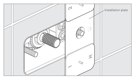
Place the installation plate over the extender, make sure that the installation plate is tight against the wall.
