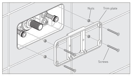
Using the four long screws and nuts, screw the trim plate down until the front of the trim plate is flush with wall, use the supplied hex key.
