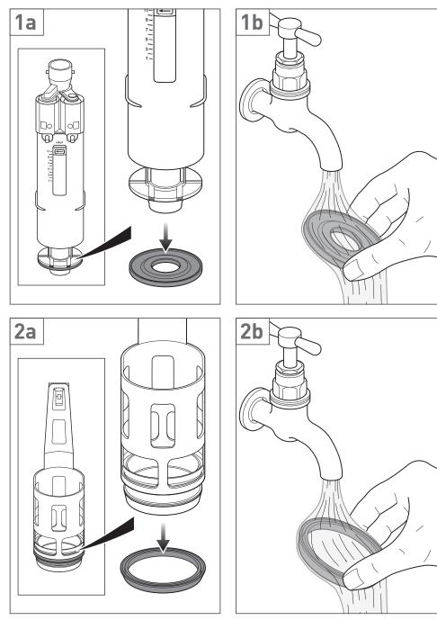
Maintenance Short Cistern WG-095A-S-F/C, WG-095A-S-C
